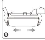
Shake the waste water tank from side to side
